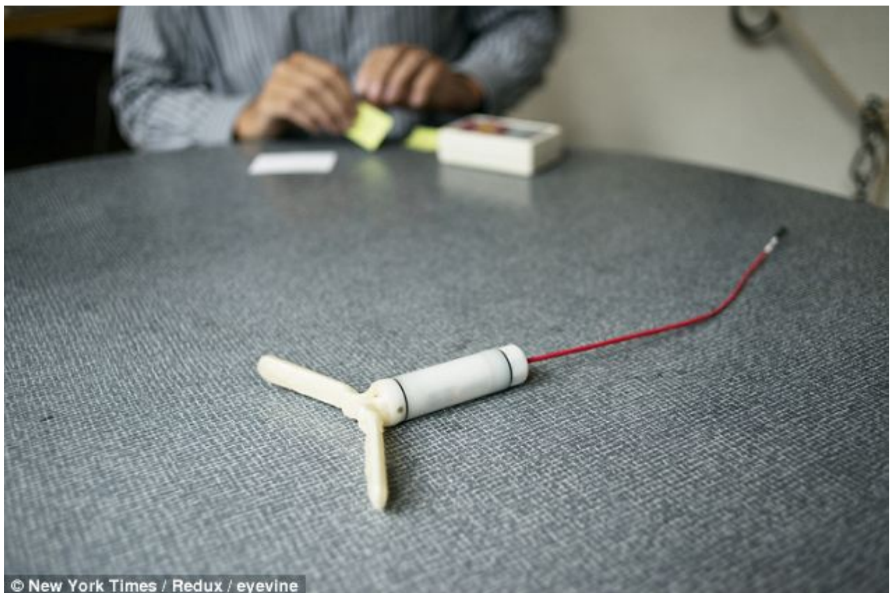
Invasive: A probe that is inserted into a cow's uterus and alerts a farmer when it is in heat. The device is being tested because the visual signs of sexual activity are harder to detect
